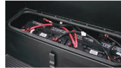
Two batteries in a single housing for easy access. (One battery in LE and Transit)
